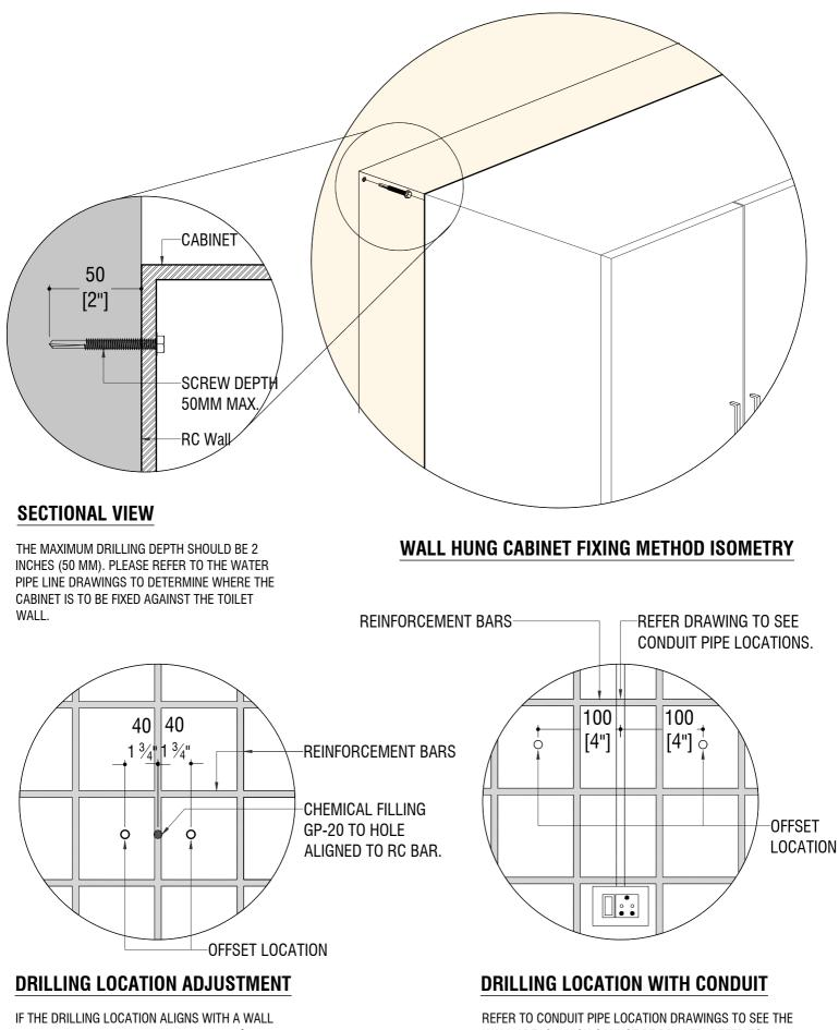
REINFORCEMENT BAR, RE-DRILL WITH A 1 <sup>3</sup>/<sub>4</sub> INCH (40 MM) OFFSET FROM THE ORIGINAL DRILLED LOCATION. IN THIS CASE, FILL THE HOLE THAT ALIGNS WITH THE RC BAR USING GP-20 HIGH STRENGTH NON-SHRINK GROUT. REFER TO CONDUIT PIPE LOCATION DRAWINGS TO SEE THE WALL AREAS WHICH CANNOT BE DRILLED.(REFER TO ANNEX.)
